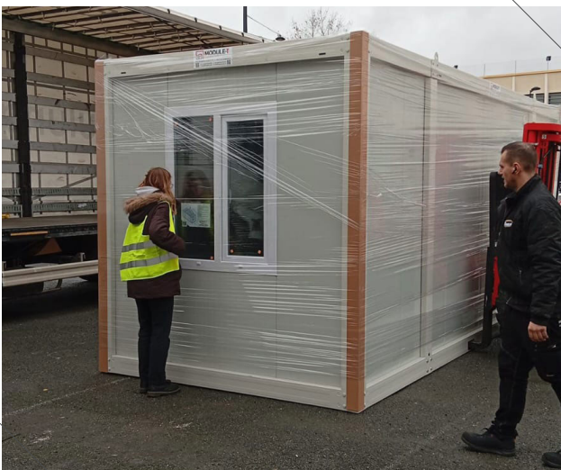
15 Wrapped module secured in trailer
