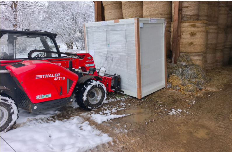
01 Winter loading of modular unit, ready to be transported to a remote worksite.
